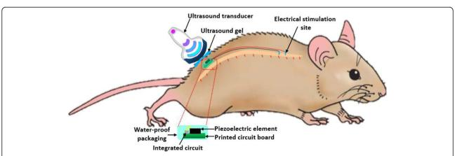
**Fig. 1** Working principle of the ultrasound-driven piezoelectric stimulator interfacing the spinal cord for the restoration of involuntary locomotion. The ultrasound energy provided by the probe is converted to electrical energy for neural stimulation by the implanted device
